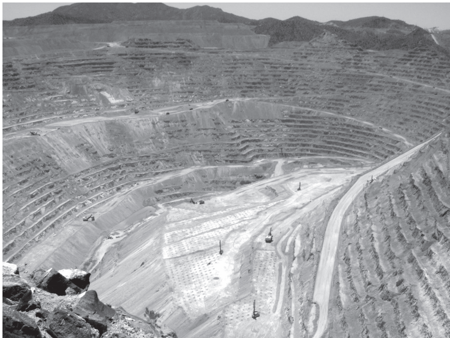
The open pit copper and molybdenum mine at Bagdad, Arizona. The deposit was located in 1882, and the open pit begun in 1945. Process facilities include a 75,000tpd concentrator, a pressure leach plant to recover molybdenum from concentrate, and an SX/EW plant that recovers up to 25 million pounds of copper annually. Presently owned by Freeport-McMoRan, the complex includes the town of Bagdad, one of the last company towns in Arizona. (Photo courtesy of Robert Spude.)
