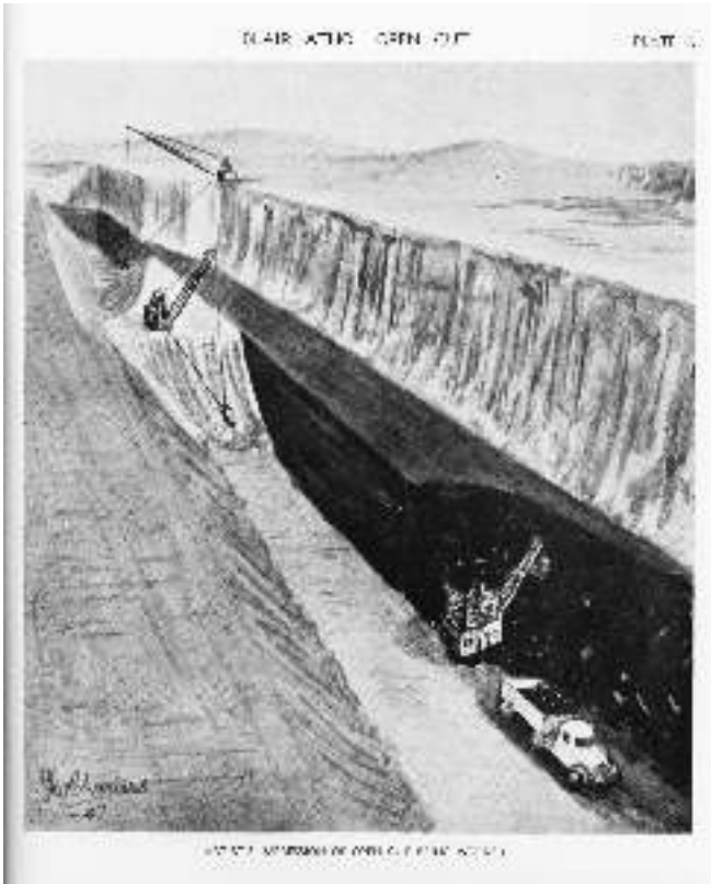
An Artist's impression of working a large-scale open cut at Blair Athol. (From Report on the Large Scale Development of Blair Athol Coalfield (Brisbane: Government Printer, 1947).)
