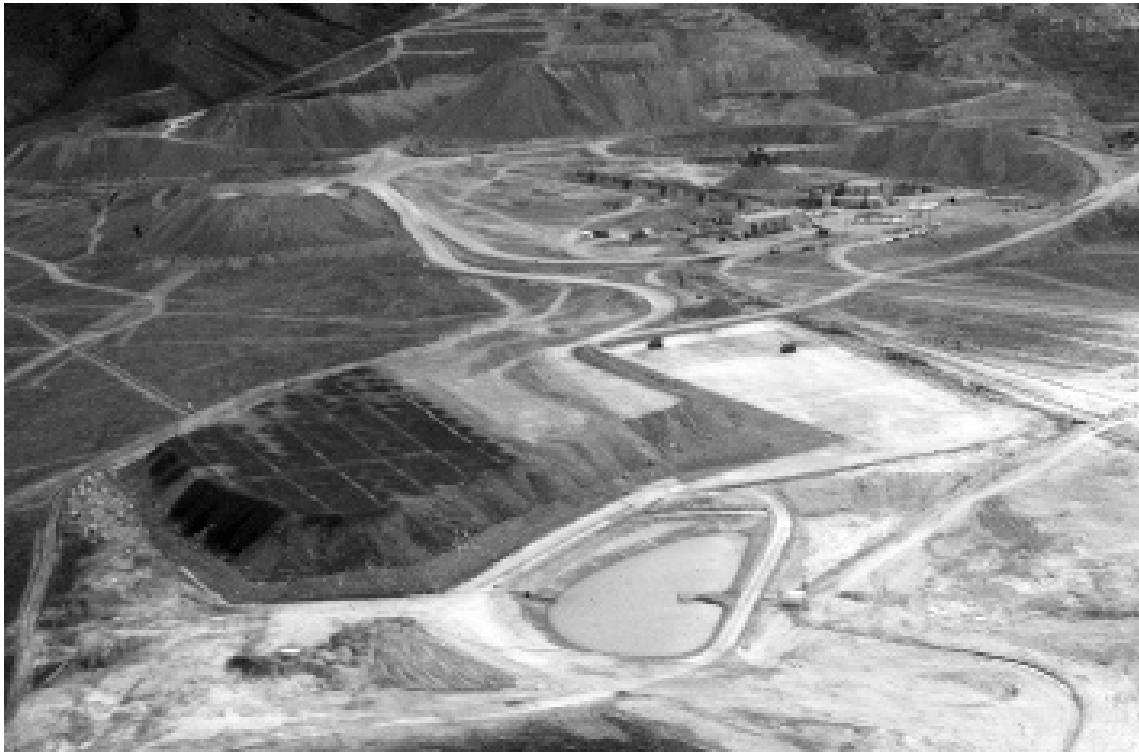
The first commercial gold recovery heap-leach pad, front left, at Cortez, c. 1971. Note the pregnant pond and recovery building in front, and equipment constructing an adjacent heap at center right. The mill and shops for the open pit operation are at upper right. (Photo by Don Duncan courtesy of Lynn Duncan.)
