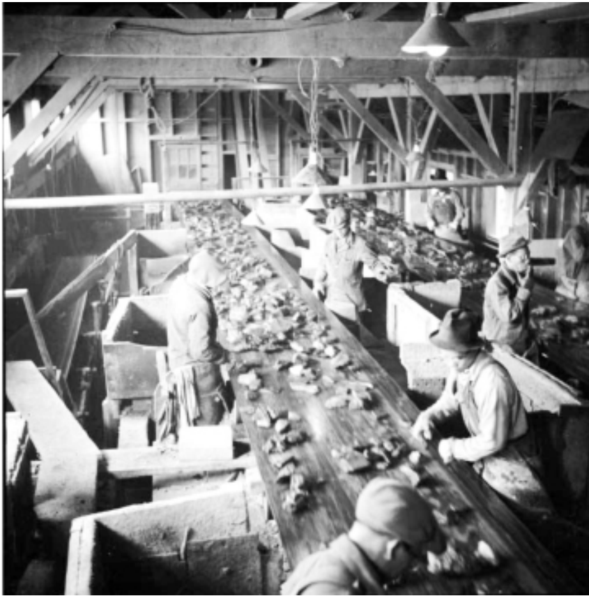
Figure 7. Filipino workers scan for quartz ore on one of the sorting decks. Ore sorting removed half of the tonnage delivered to the mill, with sorters rejecting about six thousand tons per day. Material passed by at a steady clip of 2.5 feet per second. (Evelyn Butler and George Dale Photographs, 1934-1982, Alaska State Library Historical Collections, Juneau, Alaska, ASL-P306-0271.)
