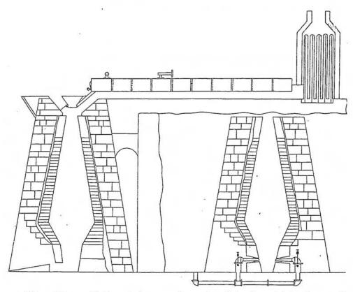
Figure 2. Diagram of Howard Furnace (Ohio) reveals the system of tuyeres introducing blasts of air into furnace to increase the temperature. (from N. W. Lord, "Iron Manufacture of Ohio" in *Economic Geology*, 1884)
