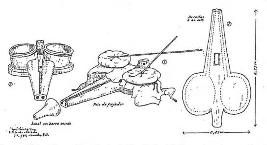
Figure 4. Diagram of Chokwe bellows used in smelting iron in Africa, showing similarities to male sexual anatomy. (from Redinha, 1953, as reprinted in Eugenia Herbert, *Iron, Gender, and Power*, 1993)
