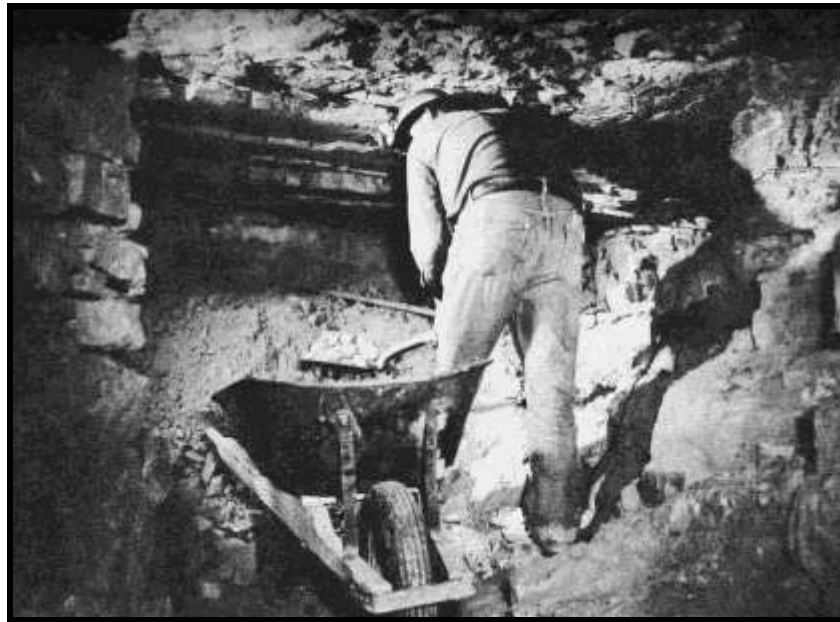
Figure E 5.10: Wheelbarrows were among the most commonly used conveyance for hauling rock out of small mines. Wheelbarrows were inexpensive and maneuverable but had a limited carrying capacity. Source: Dare: 1955:39.
