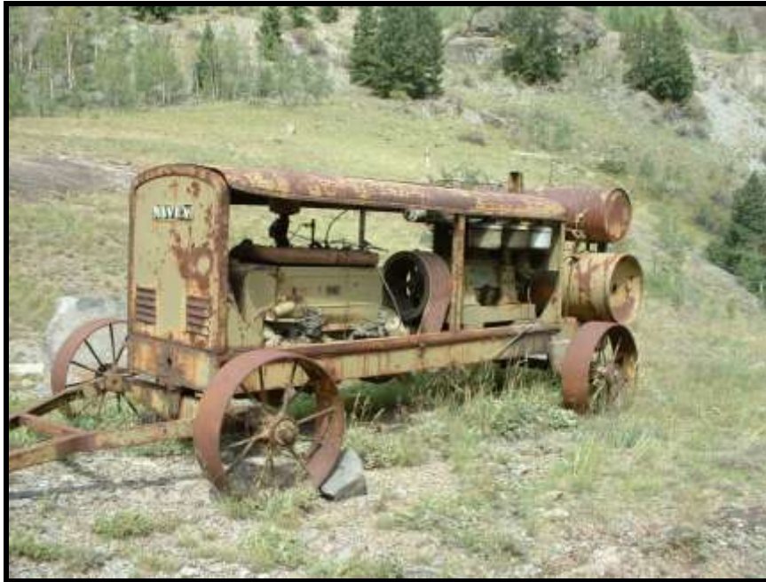
Figure E 5.13: Most uranium operations employed portable compressors instead of stationary units because of their mobility. The unit in the photo is typical of the compressors used from the 1910s through the 1930s. Source: Author.
