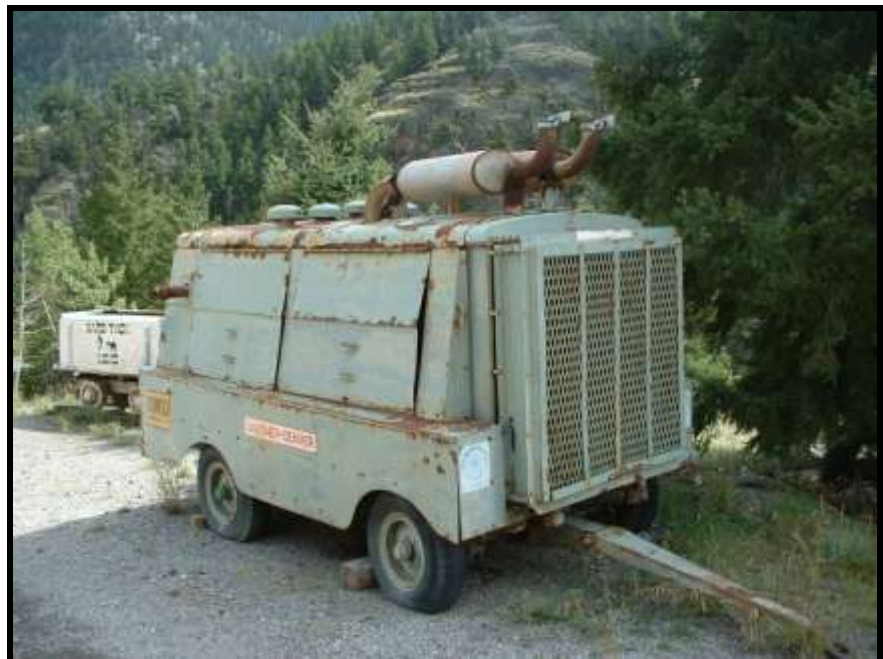
Figure E 5.14: Between the 1950s and 1970s, mining companies used portable compressors similar to the unit in the photo. Source: Author.
