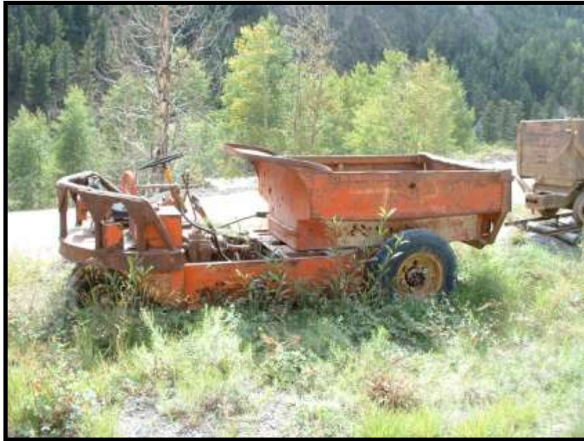
Figure E 5.12: The uranium industry began using trackless haulage vehicles during the 1950s. The vehicles replaced ore cars, required no tracks, and allowed miners to haul out more rock. Source: Author.
