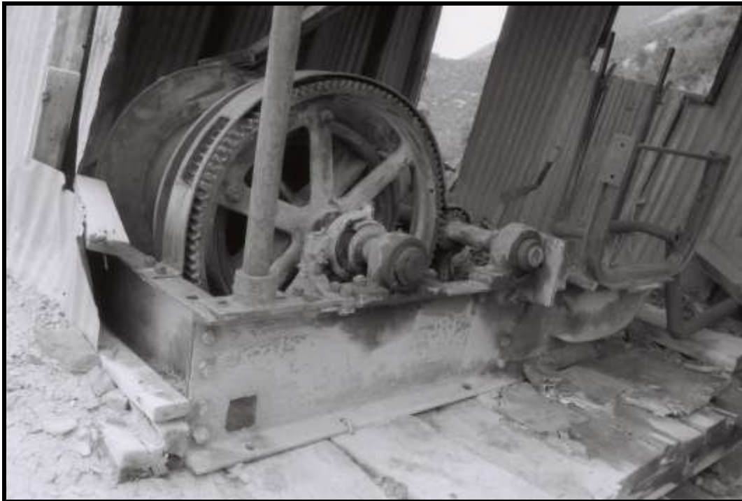
Figure E 5.24. The Mary Ann Mine on Davis Mesa featured a factory-made gasoline hoist. The cable drum, left, and engine mount, right, were bolted to a steel frame. The engine, now gone, turned the drum via the reduction gearing. Source: Author.
