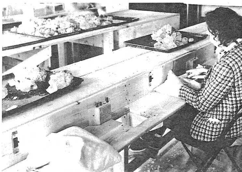
Fig. 15 Crystal Shop. Final inspection and cobbing station.
