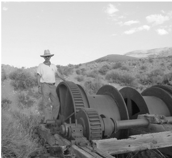
Hoisting drums at Cornucopia. Photo courtesy of Summit Envirosolutions, Inc.
