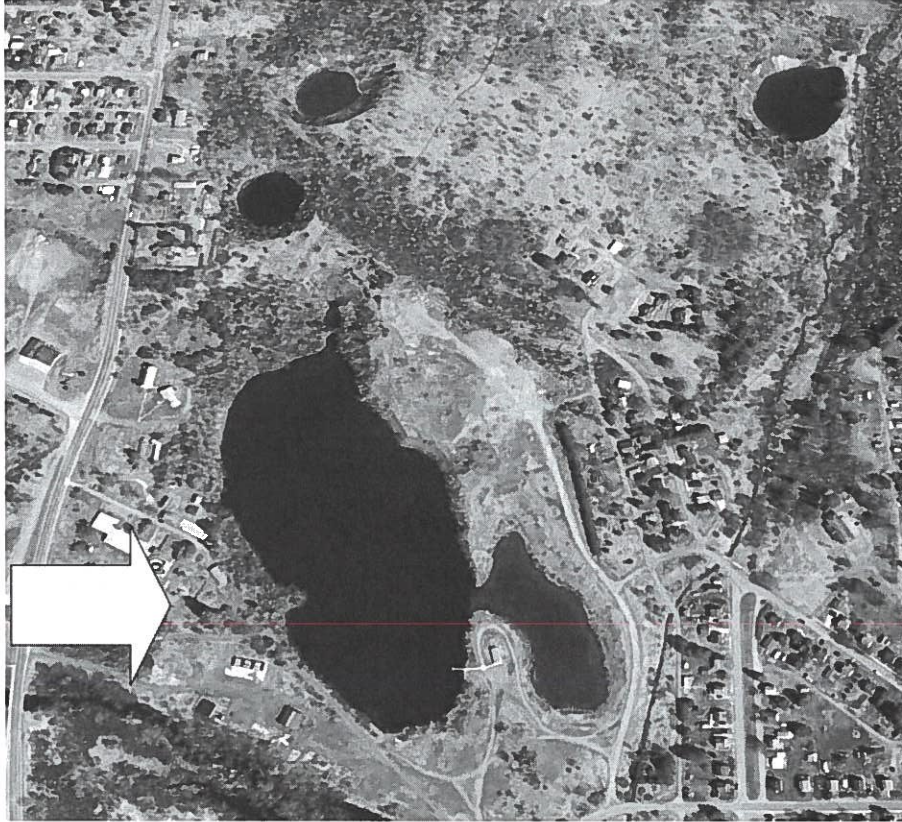
The large, flooded subsidence at the Caspian mine -- note additional caving ground to the north and northeast. (Arrow denotes site of Caspian No. 1 headframe and museum.)
