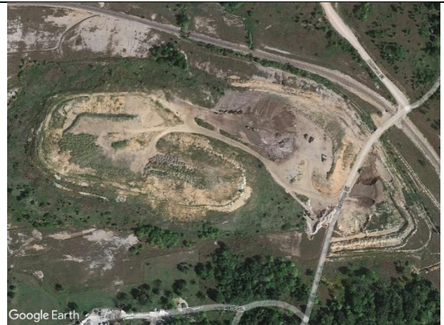
The "Hells Half Acre" mine subsidence area, across Route 66 from the Galena Smelter, has been reclaimed through Superfund and is being repurposed as a landfill.
